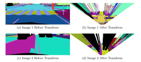
Figure 6: Examples of the homography transform applied to the output of the segmentation camera (the recoloring can be ignored, its due to the conversion between BGR to RGB)
