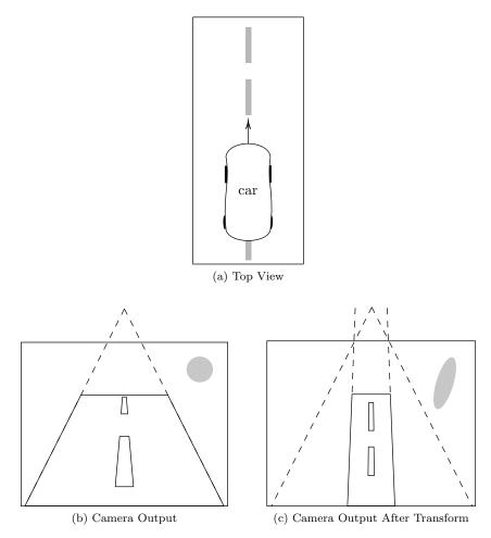
Figure 5: Application of the homography transform on an image to fix the perspective of the camera on the road
