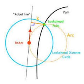
Figure 3: A visualization of the perpendicular distance of the car to the goal point. The goal point is colored green and the perpendicular distance is labeled as X colored in orange
