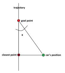
Figure 3.5: A visualization of the closest point, the goal point and the car's position connected as a triangle. Note the closest point is coined as "closest" because the closest point on the trajectory from the car's position is defined to be the perpendicular line connecting the segment to the car's position
