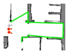
Figure 1: The Monte Carlo Localization (MCL) algorithm in action. Notice how the first particle (one possible odometry of the car) is eliminated because its lidar beams (the green shape) is ruled as unlikely. The middle particle will be ruled as most probable, hence it'll be kept as the most probable odometry.
