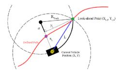
Figure 2: A visualization of the closest point on the trajectory (marked purple), the goal point (marked green) and the global position of the car (marked yellow).
